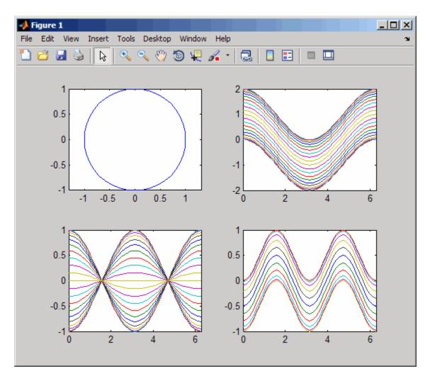
Each subregion contains its own axes with characteristics you can control independently of the other subregions. This example uses the axis function to set limits and change the shape of the subplots.
