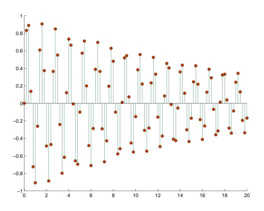
You can generate code to reproduce this graph by selecting **Generate code** from the **File** menu. MATLAB code generation software composes a function that recreates the graph and opens the generated file in the editor.
