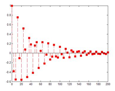
Setting the aspect ratio of the *x*- and *y*-axis to 2:1 improves the utility of the graph. You can do this by setting the aspect ratio of the plot box using pbaspect:
