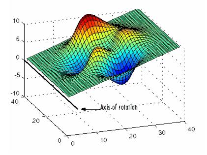
Notice that the surface rotated -15 degrees about the *y*-axis that passes through the origin. However, to rotate about the *y*-axis that passes through the point x = 20, you must translate the surface in *x* by 20 units.
