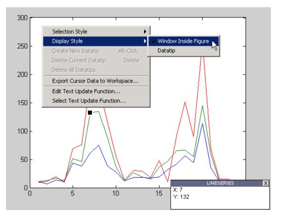
**Note** If you change the data cursor **Display Style** from **Datatip** to **Window Inside Figure** with the context menu, only the most recent data tip is displayed; all other existing data tips are removed because the window can display only one datatip at a time.
