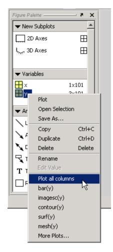
For example, the following picture illustrates how to plot the columns of variable Z. This is equivalent to passing a matrix to the plot function.
