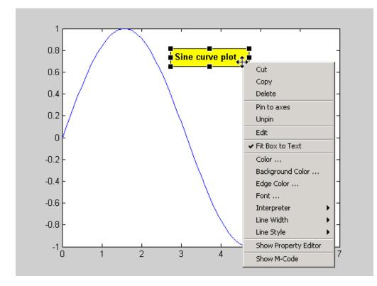
When you create a textbox without dragging it to have a specific size, **Fit Box to Text** is enabled, and the box will grow or shrink as you type or edit its text. If you drag when creating a textbox, or change its size by dragging any of its handles in plot edit mode, **Fit Box to Text** is disabled, but you can re-enable it using the context menu.
