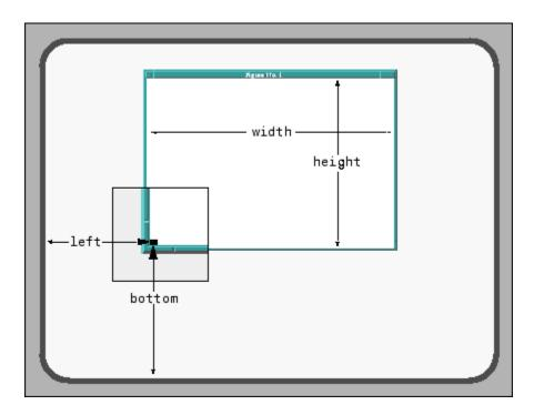
MATLAB does not measure the window border when placing the figure; the **Position** property defines only the internal active area of the figure window.
