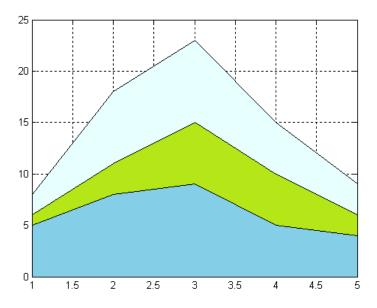
**Displaying the Grid on Top.** To display the grid lines in the foreground of the area graph and display only five grid lines along the *x*-axis, use the statements
