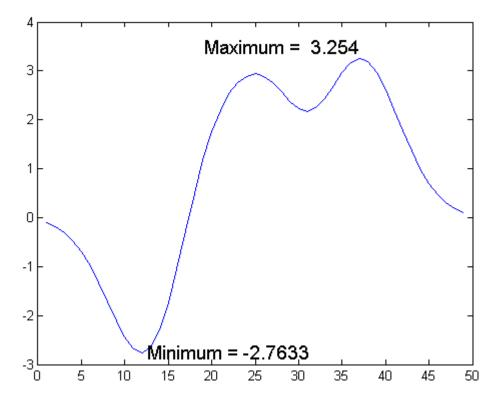
The text function positions the string relative to the point specified by the coordinates, in accordance with the settings of the alignment properties. For the minimum value, the string appears to the right of the text position point; for the maximum value the string appears above and to the left of the text position point. The text always remains in the plane of the computer screen, regardless of the view.
