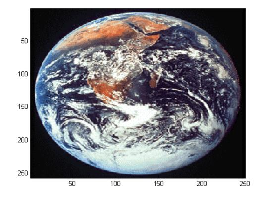
The elongated globe results from stretching the image display to fit the axes position. Use the axis image command to force the aspect ratio to be one-to-one.
