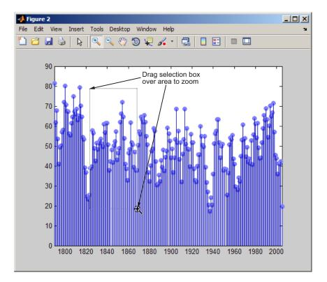
results in a rescaling of the axes to display only that region.
