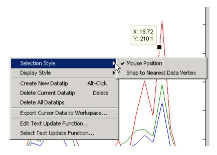
MATLAB does not honor interpolation mode when you use the arrow keys to move a datatip to a new location.
