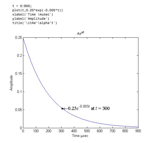
To annotate the point where the value of t = 300, calculate the text coordinates using the function you are plotting.
