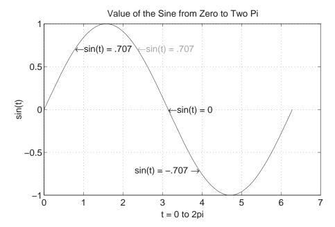
Suppose you want to move the text string labeling the value sin(t) = .707 from its current location at [pi/4, sin(pi/4)], to the point [3\*pi/4, sin(3\*pi/4)] where the function has the same value (shown grayed out in the picture). To do this, determine the handle of the text object labeling that point and change its Position property.
