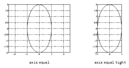
If you want the axes shape to conform to the plotted data, use the tight option in conjunction with equal.
