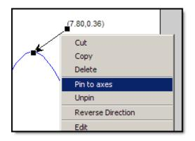
The black handles of the arrow become hollow to indicate that the object has been pinned.
