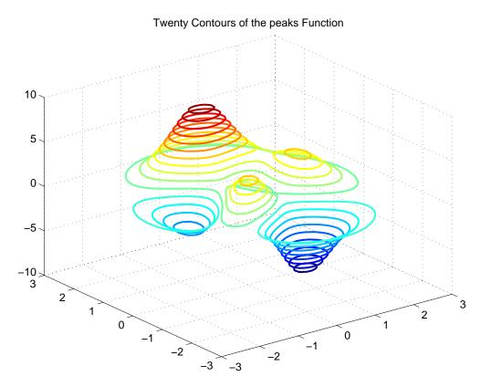
display 20 contours of the peaks function in a 3-D view and increase the line width to 2 points.
