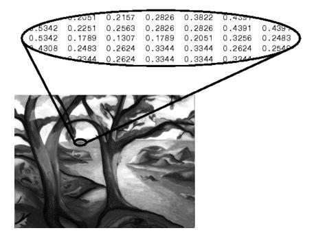
To display an intensity image, use the imagesc ("image scale") function, which enables you to set the range of intensity values. imagesc scales the image data to use the full colormap. Use the two-input form of imagesc to display an intensity image, for example:
