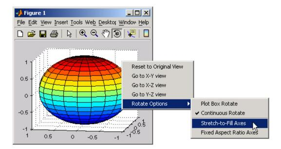
The next picture shows how the **Fixed Aspect Ratio Axes** option results in a sphere that maintains its proper shape as it is rotated.
