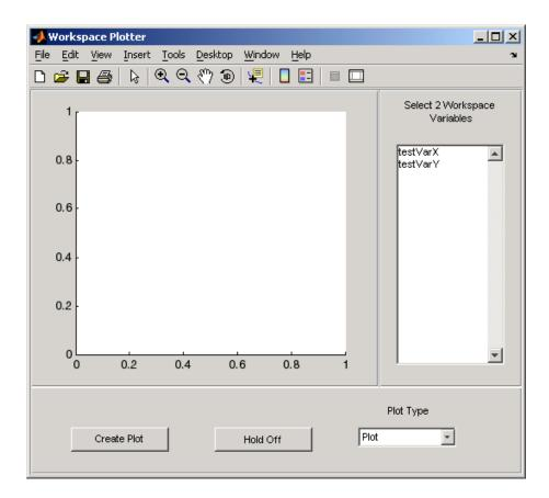
The GUI layout is split among three uipanel containers. The left-hand panel contains the axes, the right-hand panel contains a list box to display workspace variables, and the bottom panel contains the plot and hold buttons and the plot type pop-up menu.
