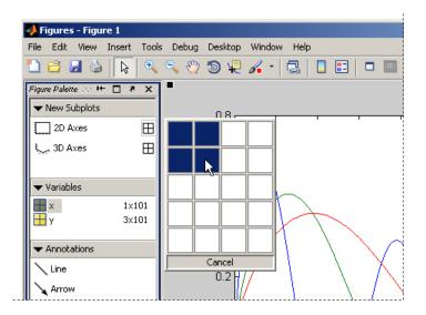
The picture above shows the **New Subplots** panel selected to display four equally sized axes in the figure. Existing axes resize as required to accommodate the new layout.
