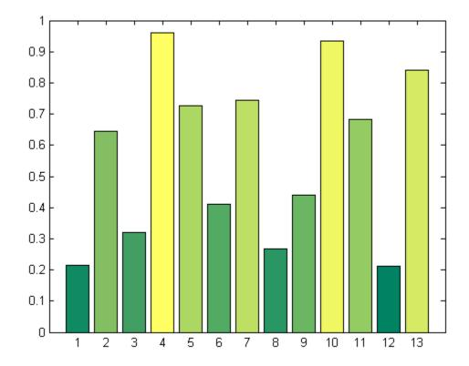
The code assigns colors to bars based on their YData ranks, rather than on their YData values. This helps to distinguish bars by color, but also the code can assign to bars that are nearly the same height a wider range of colors than if the colors were directly mapped to YData values.
