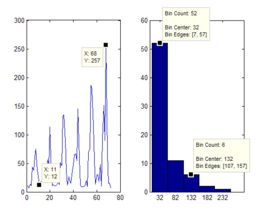
When you add datatips to histograms or bar graphs showing groups of data, you can move a datatip to any other bar by clicking inside that bar. If you use the cursor keys to shift a datatip back or forth across the graph, the datatip moves to the preceding or succeeding bar of the same color.
