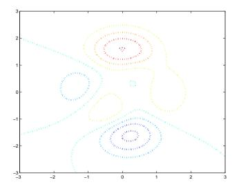
The contour plot object lets you set the line width and style of the contour graph by setting two properties. Looking at the core objects contained in the contour plot object reveals a number of patch objects whose edges are used to implement the contour line, which you would otherwise need to set individually.
