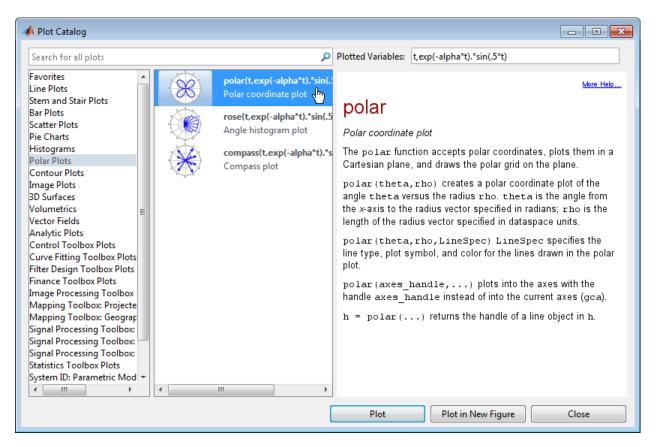
The following picture shows the Plot Catalog tool with the polar graphing function selected to display the expression t,exp(-alpha\*t).\*sin(.5\*t).
