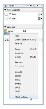
5 When the Plot Catalog tool opens, add the expression to the Plotted Variables text field so it reads t, exp(-alpha\*t).\*sin(.5\*t). You can reference the variable alpha because you created it in the base workspace.
