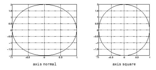
The square axes has one data unit in *x* to equal two data units in *y*. If you want the *x*- and *y*-data units to be equal, use the command
